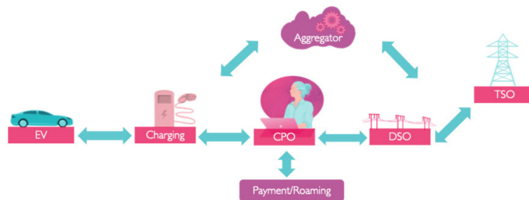
Image 3: Electric car, aggregator, DSO, TSO, charger, and service operator are all parts of a system that needs to communicate with each other.
